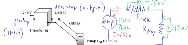
a) Calculate the number of turns required on the primary winding.
